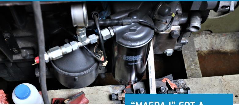
Initially, there were a few issues to resolve. The engine shell was too high. It was necessary to disassemble it, shorten and reassemble in order to align the engine with the propeller shaft line. Fortunately, we found the right weather, because the resin should cure in the temperature range of 15 - 25 degrees Celsius.
